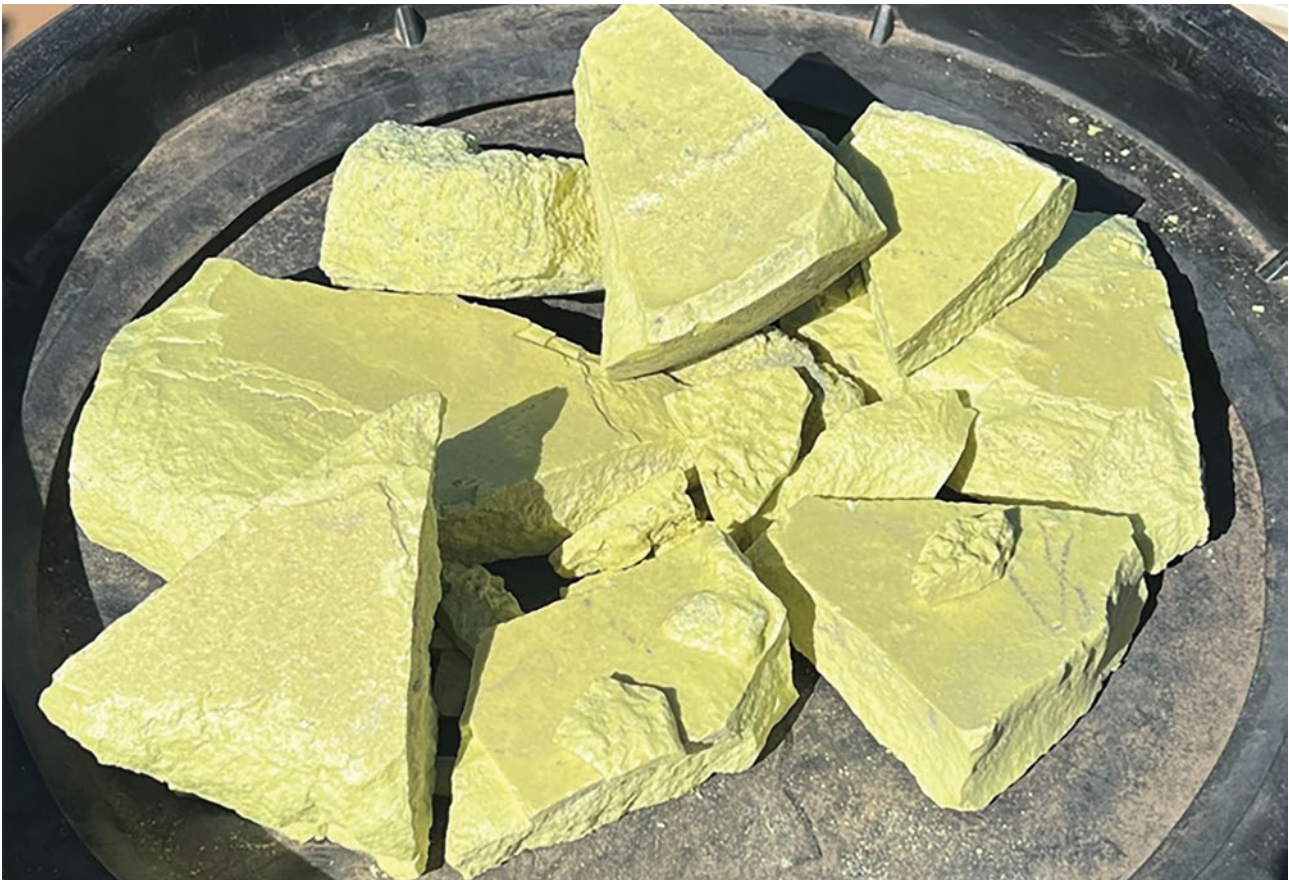
Figure 3 – Elemental sulphur produced from the calcining of concentrate in the kiln
