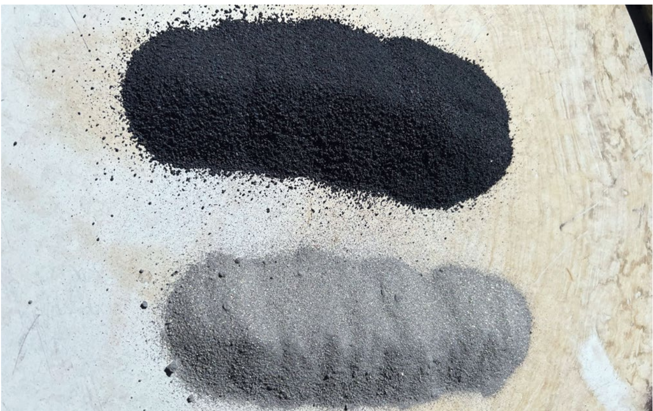
Figure 2 – Comparison of BHCP dry concentrate (grey) and magnetic fraction of the calcine (black)
