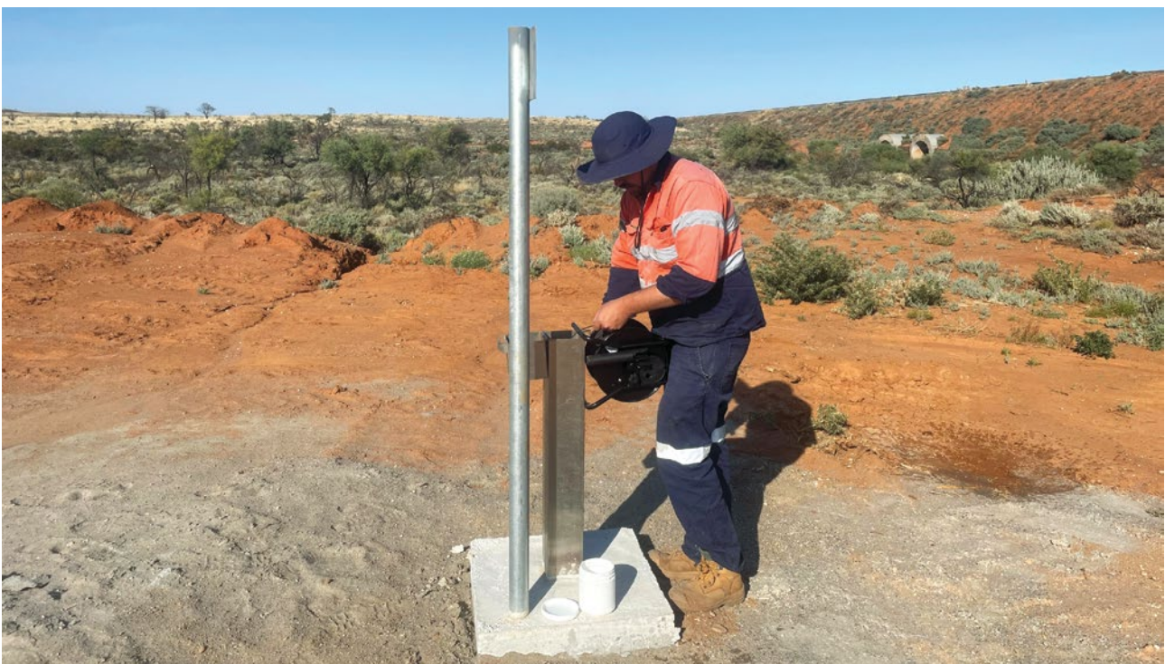
Figure 9 – BHCP geologist undertaking groundwater measurements
