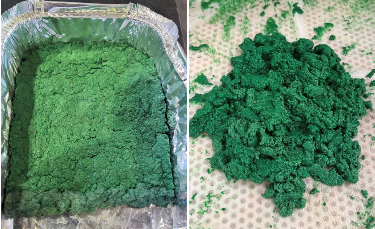
Figure 5 – First batches of Mixed Hydroxide Precipitate (MHP) from the BHCP Demonstration Plant
