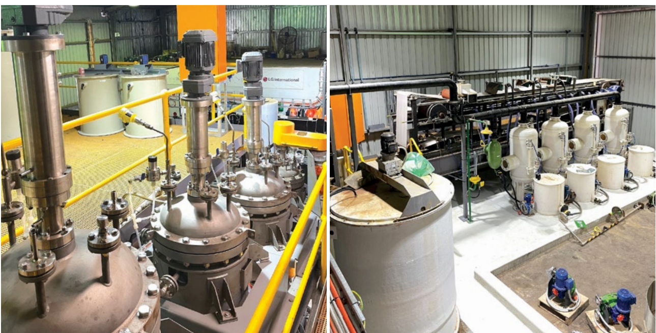
Figure 4 – Horizontal vacuum filter belt and Pressure oxidation leach circuit
